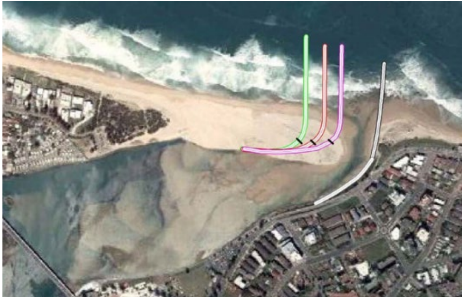
Figure 2.5: Training walls investigated by Cardno 2013.
