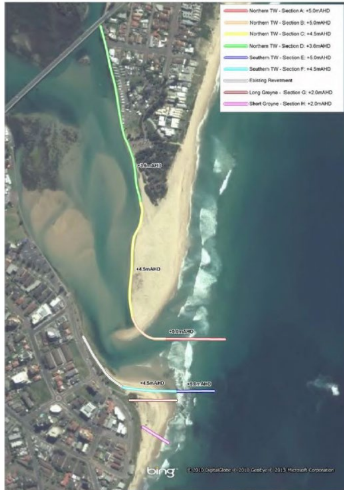
Figure 2.7: Fully trained entrance wall at the Entrance channel, reprinted from (GHD, 2019).
