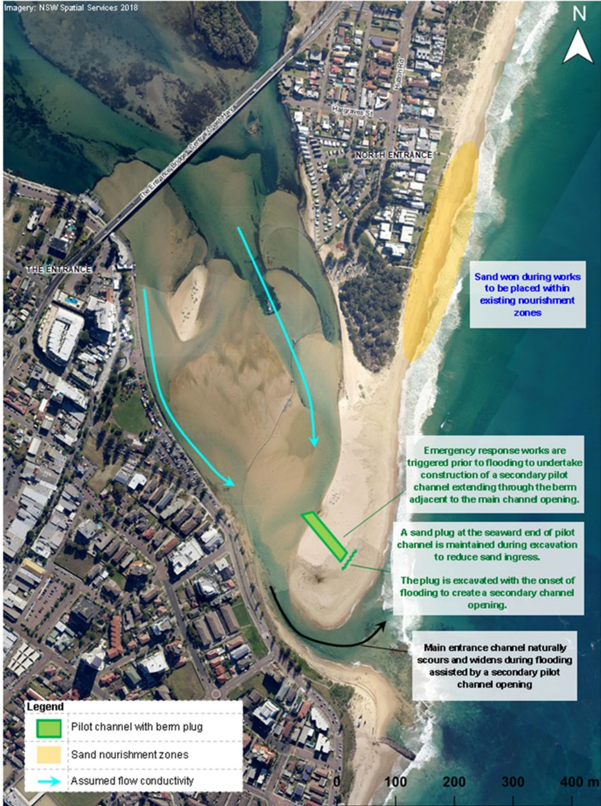
Figure 4.1: Option 2 Emergency pilot channel opening shown for open entrance in a constricted state
