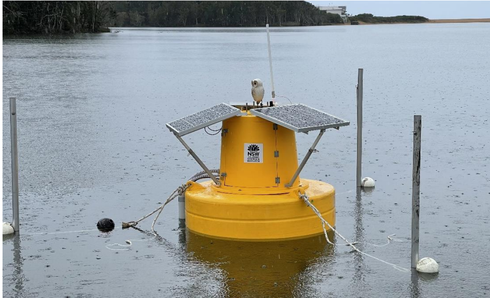
Figure 5. Beatrice the smartbuoy, a telemetered water quality buoy on Avoca Lagoon (Nov 2021)
