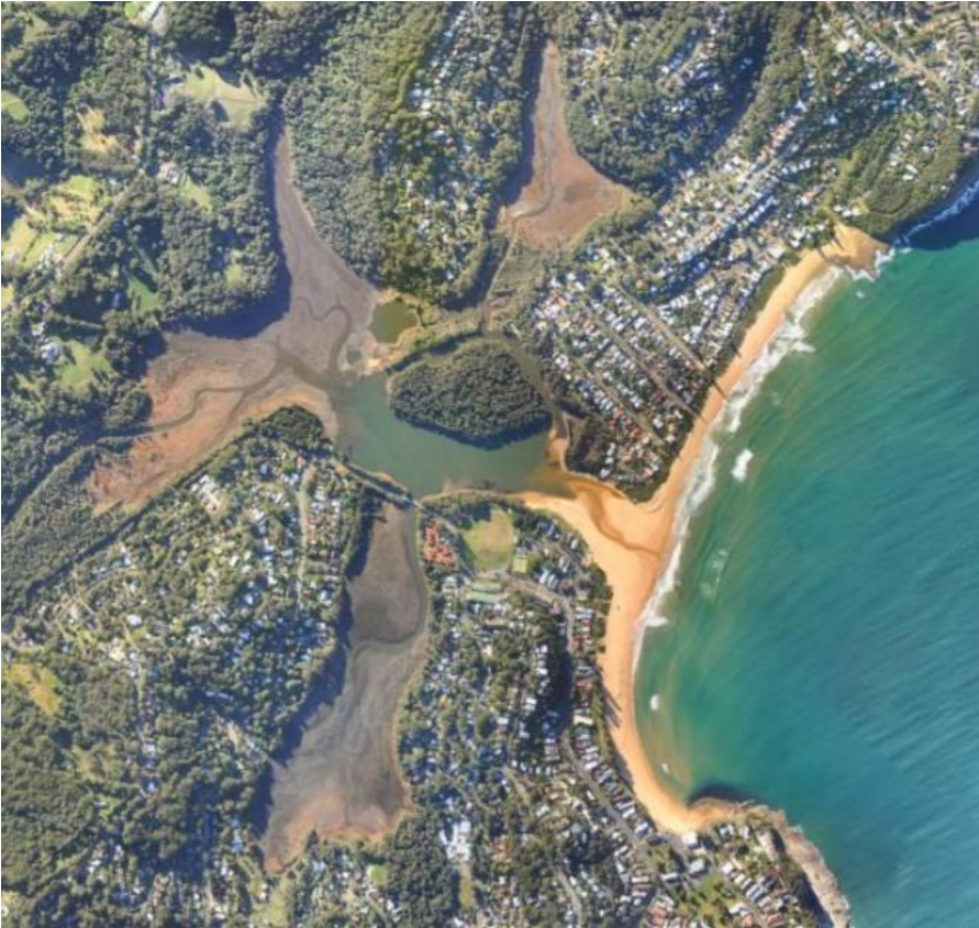
Figure 3. Aerial image of Avoca Lagoon from 2012 clearly showing the dredge hole in the central basin (Nearmap, 2024)
