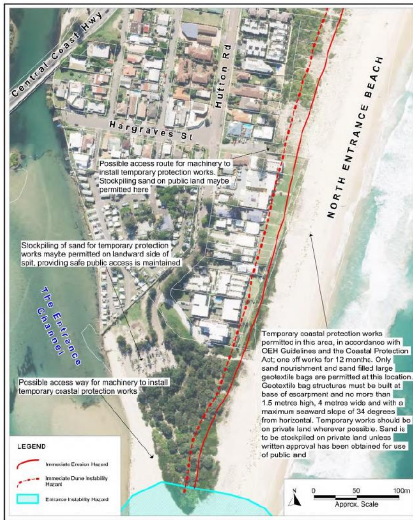
Figure 36: Temporary Coastal Protection Works Options for Private Property at Entrance North Beach – Hutton Road (BMT WBM, 2018)
