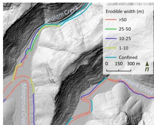
**Figure 8.** Example of streambank delineated by erodible width
