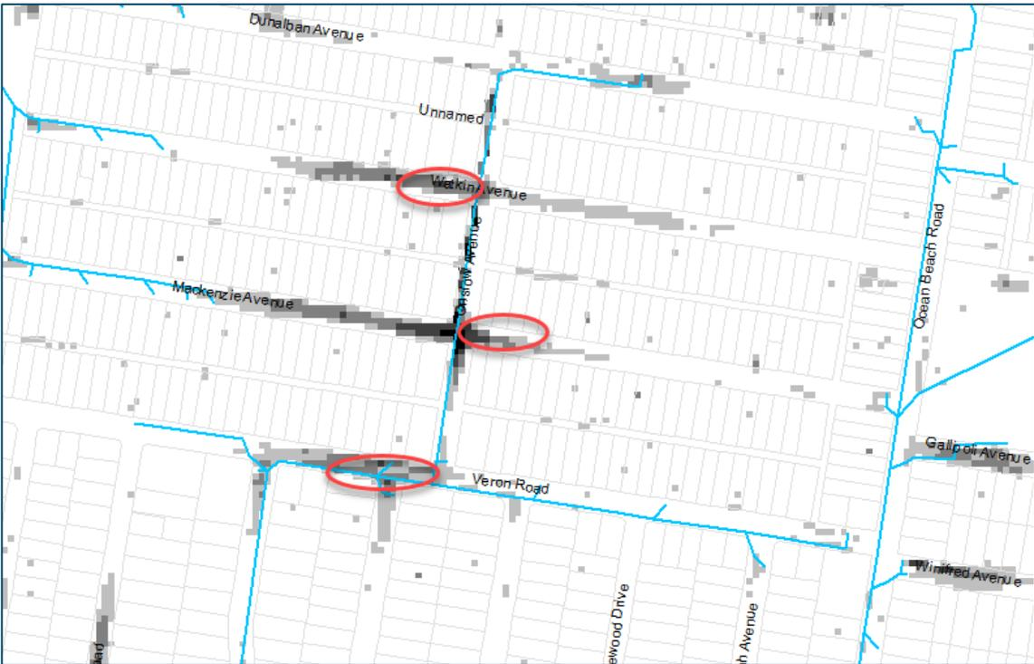
Figure 13.4 FM03 nominated locations for infiltration devices in the area with relatively shallow sand layer
