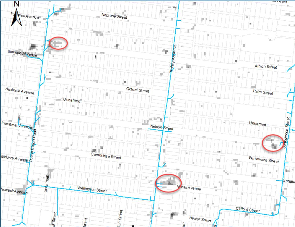
Figure 13.3 FM03 nominated locations for infiltration devices in the area with relatively deep sand layer
