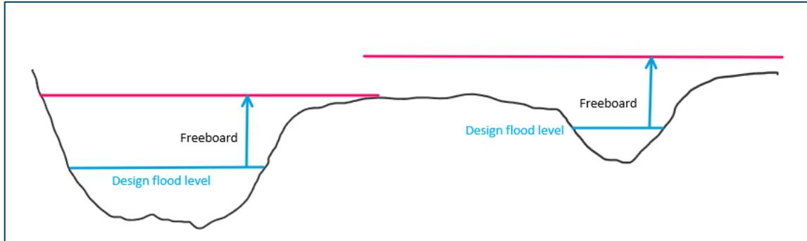
Figure 10.3 Different Flood Planning Level from two separate flood areas
