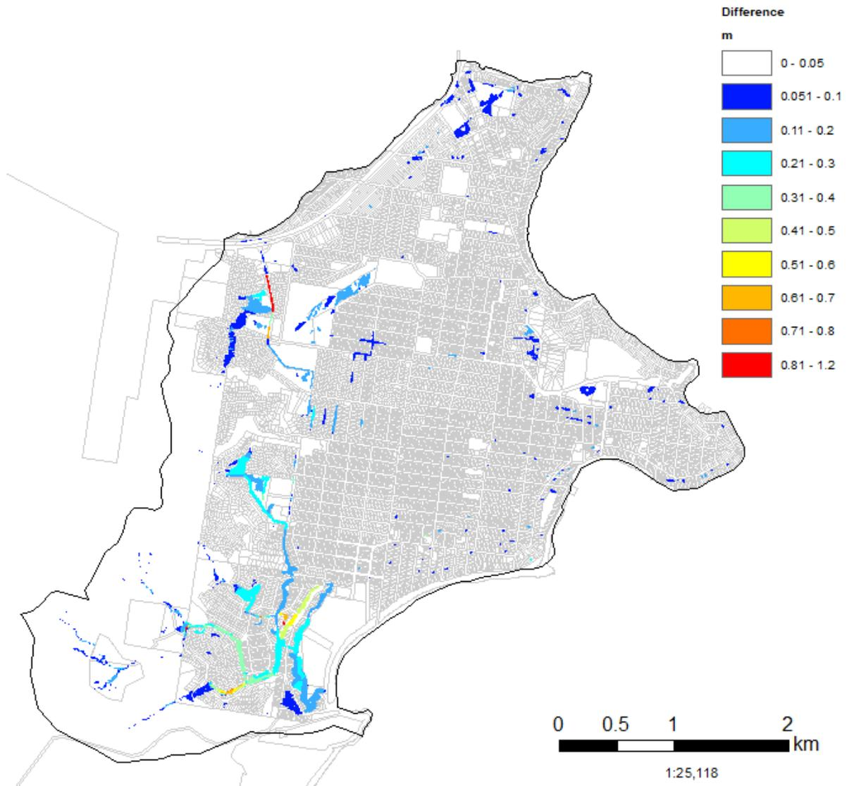
Figure 10.6 Difference in Flood Levels of 1%AEP versus 30% Rainfall Intensity Increase and 1%AEP
