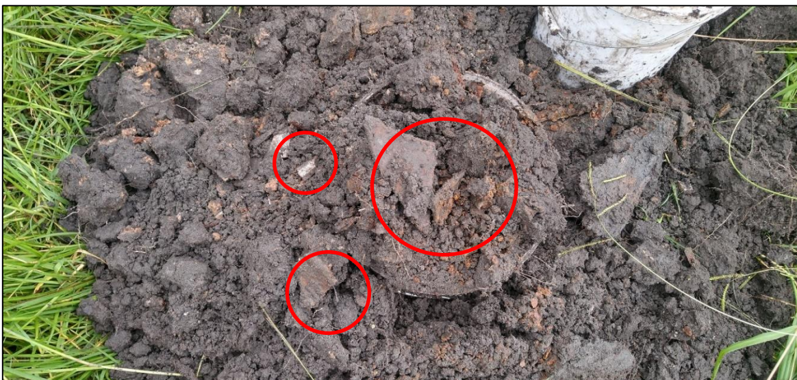
Figure 6: Fibrous cement material (circled) observed in a test pit excavated in the asbestos delineation area.
