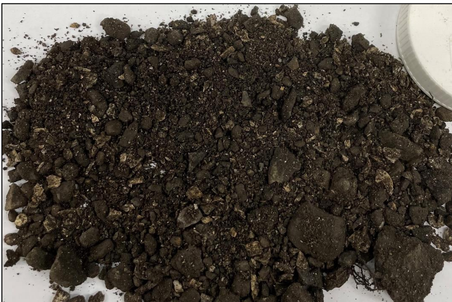
Figure 10: Carbonaceous (i.e. ash, charcoal or residual material from fires) material observed in Sample 128/0.1
