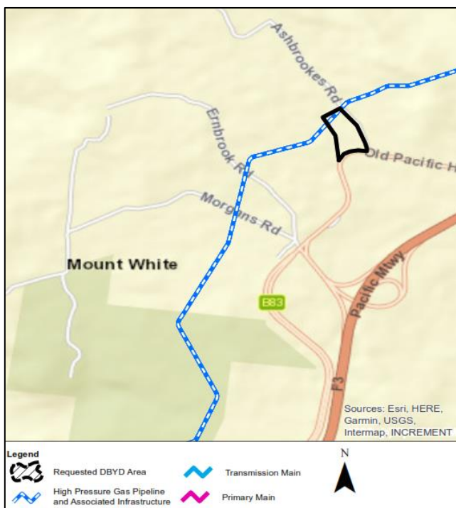
Figure 2: Alignment of high pressure gas (and fuel) pipeline intercepting the northern portion of the site (outlined in black). Figure extracted from Jemena Gas Networks DBYD search.
