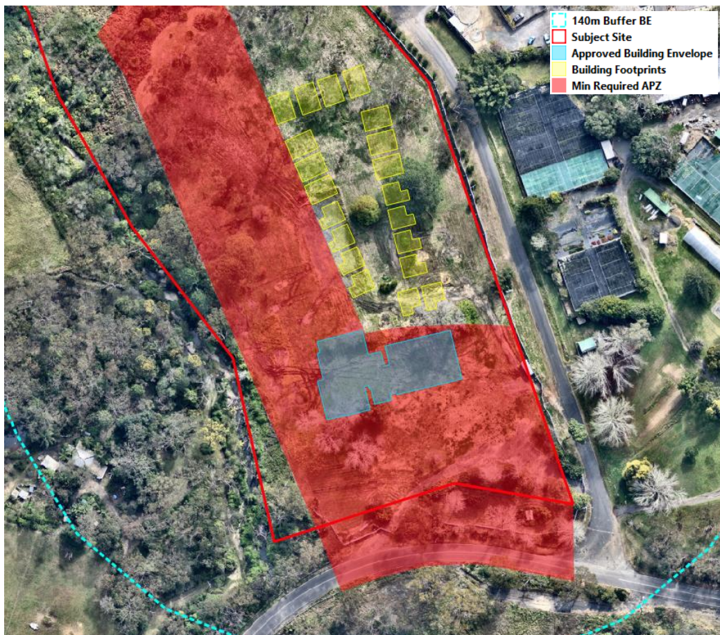
Figure 06: Aerial image of the subject site overlaid with the minimum required APZs from new SFPP development (red shade)
