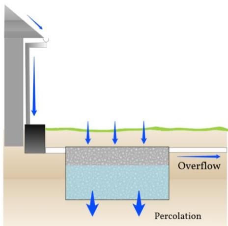
Figure 6.4 Option 3 – Example sketch of detention tank in residential area to increase storage at allotment scale
