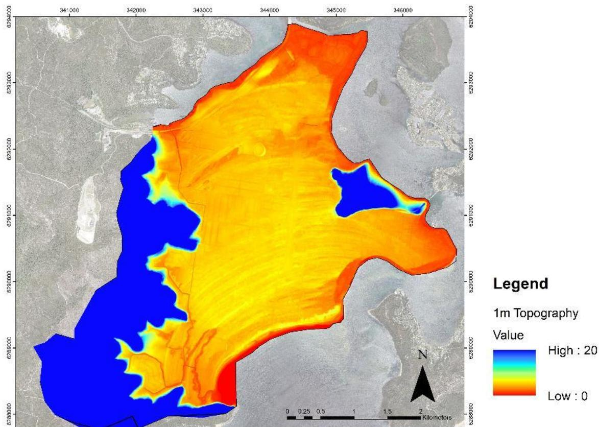
Figure 2.1 1m grid topography processed from LiDAR
