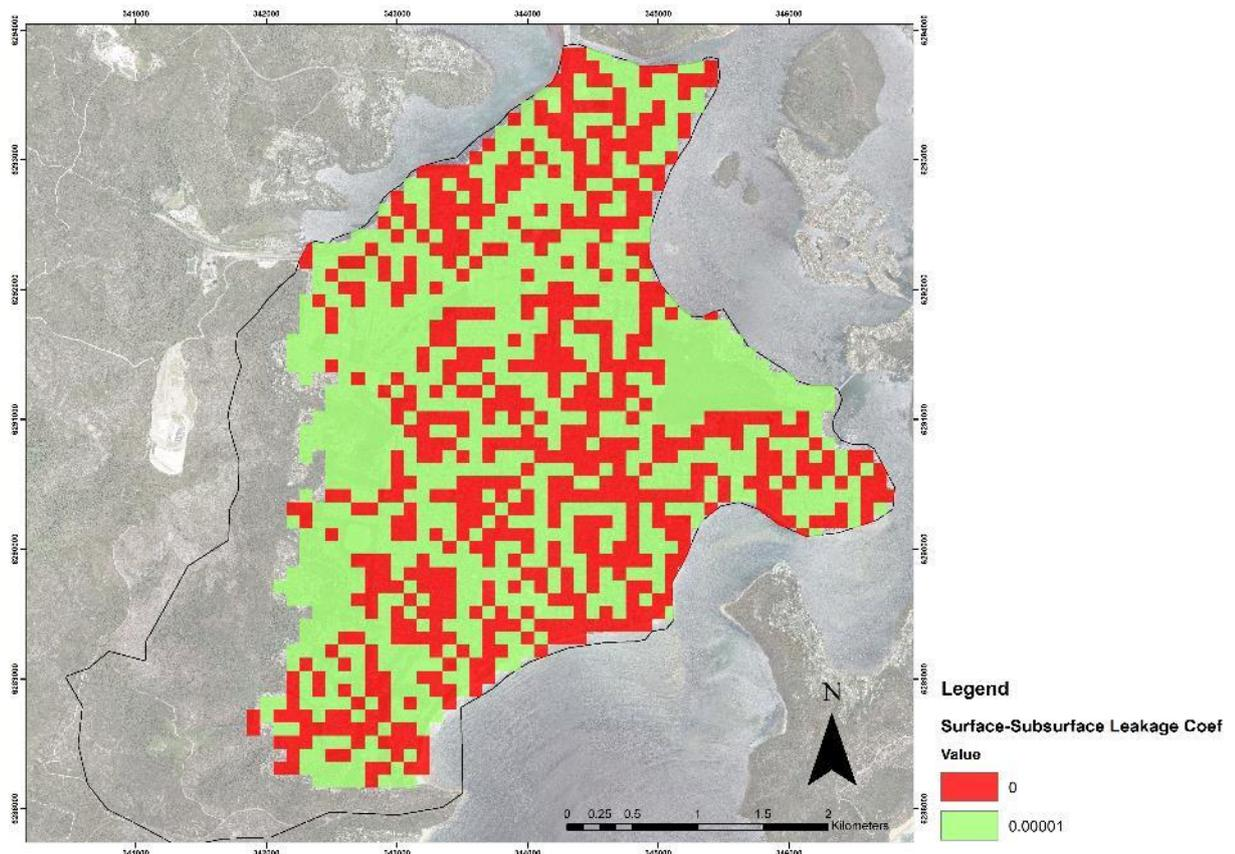
Figure 4.1 Surface-subsurface leakage coefficient
