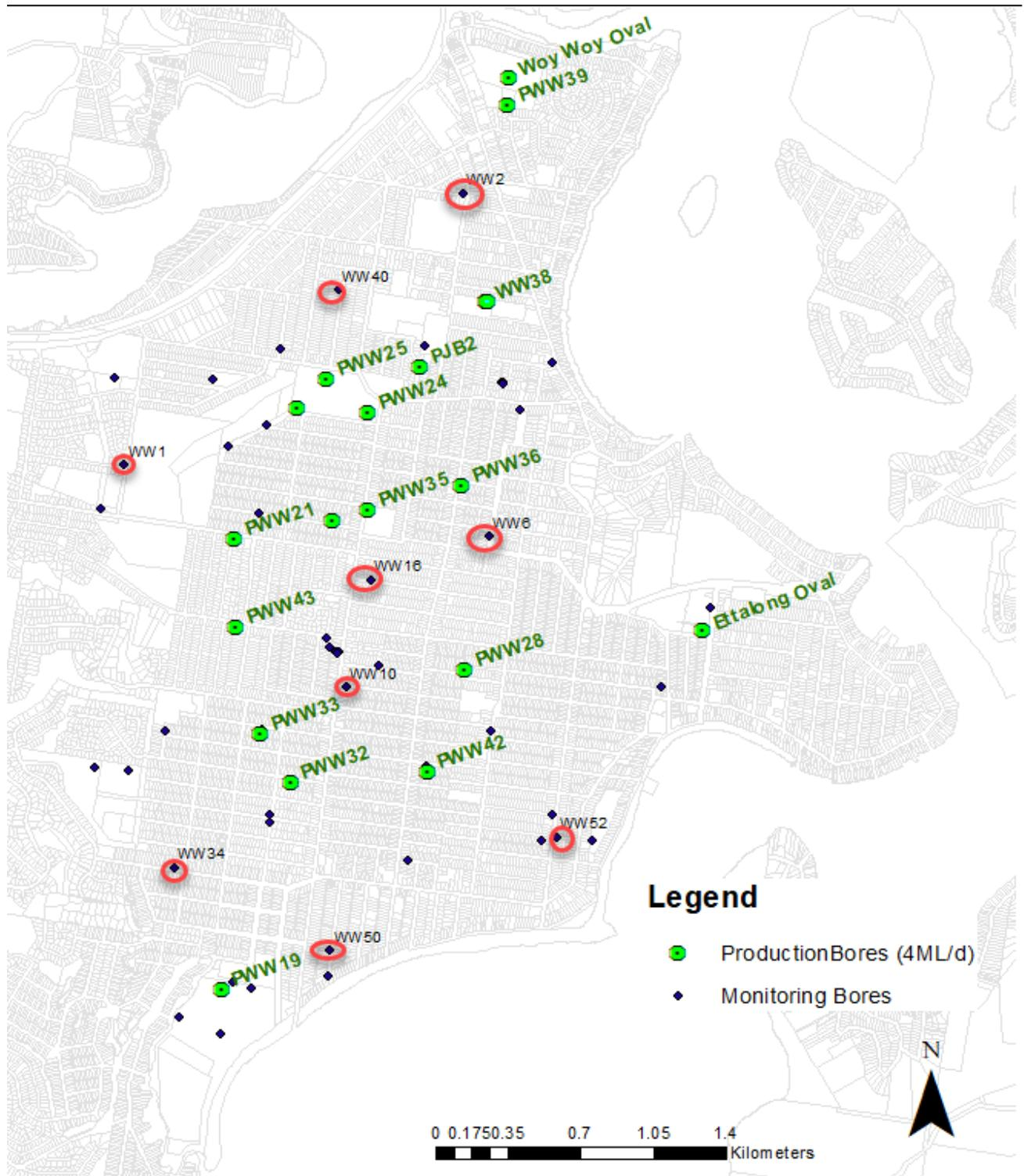
Figure 5.1 Production Bores for portable and recreational purposes and Monitoring Bores
