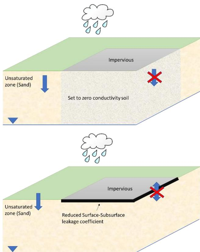
Figure 3.5 Representation of an impervious area in the existing model (top) and in the updated model (bottom)
