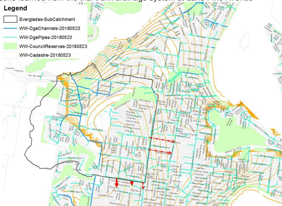
Figure 6.2 Option 1 Conceptualisation: Stormwater runoff is redirected towards the east (indicated by red arrows), following the natural groundwater gradient. The Everglades Catchment is outlined in black, example groundwater contours are shown as orange lines.
