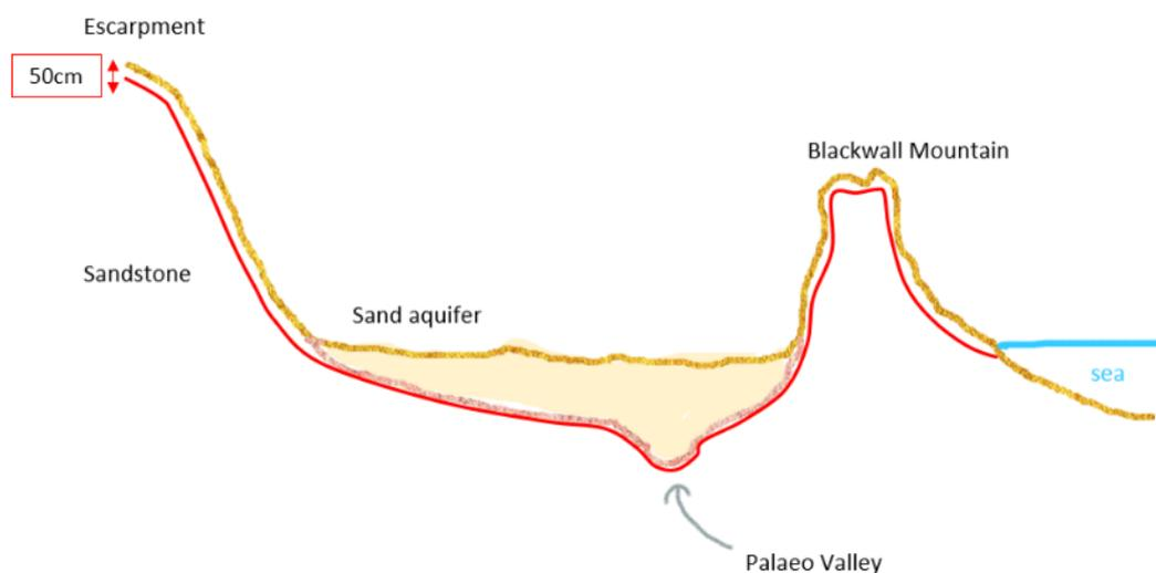
Figure 3.4 Schematic of a typical west-east cross section of the Woy Woy peninsula (red line: the bottom of the saturated zone layer 1 in the model)
