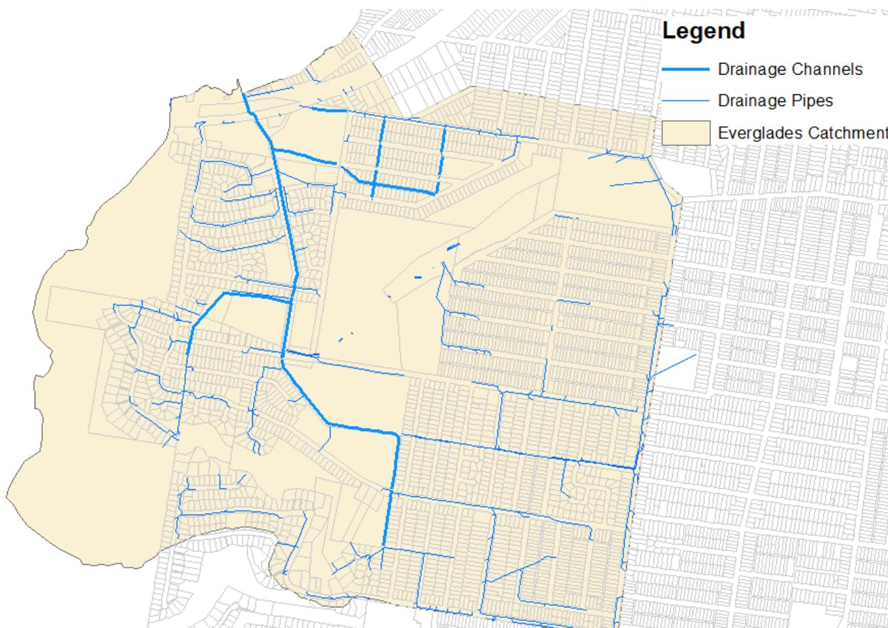
Figure 6.1 Drainage pipes and channels in Everglades Catchment
