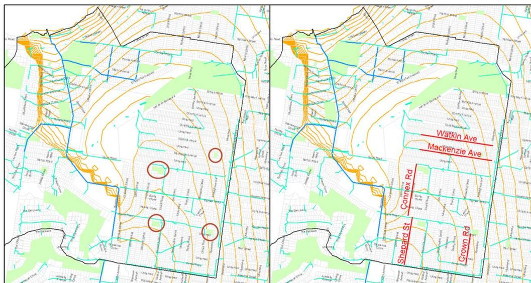
Figure 6.3 Option 2 – Potential locations for water storage (left, indicated by red circles) and exfiltration pipes (right)
