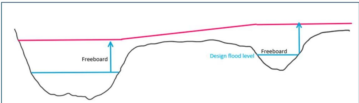
Figure 10.5 Flood Planning Level interpolated from two separate design flood levels
