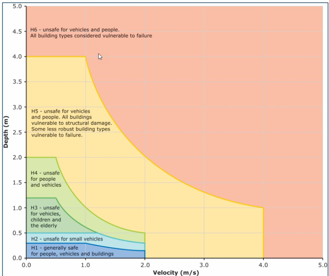
Figure 8.5 Combined Flood Hazard Curves (Smith et al., 2014) (Figure 6.7.9. of ARR 2016)
