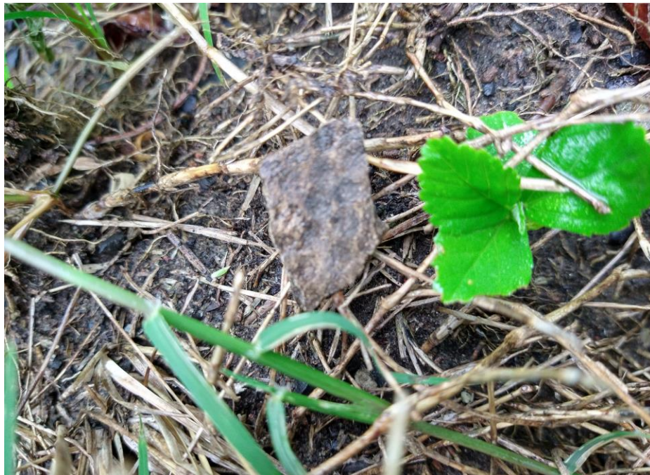
Photo 6 – Fragment of potential asbestos containing material on ground surface
