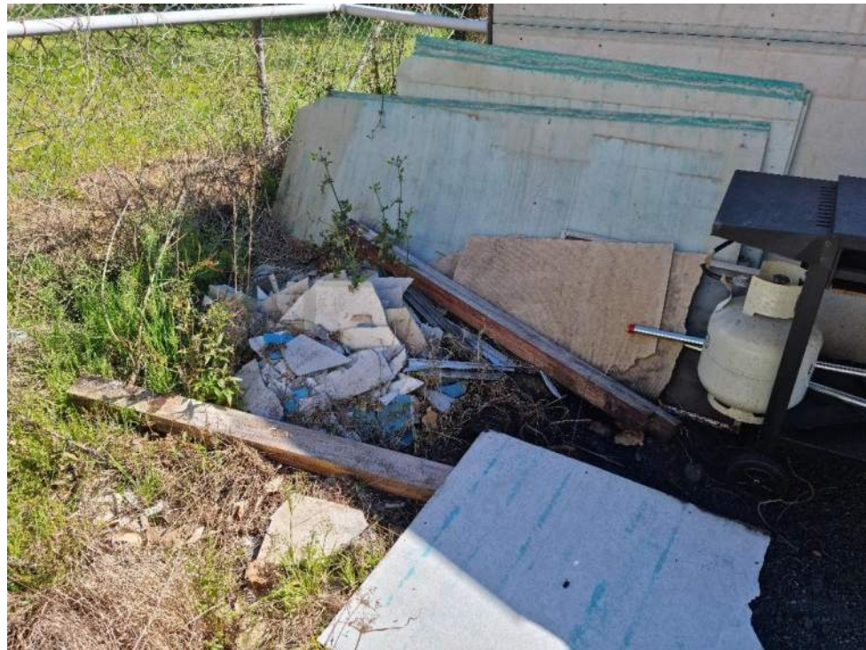
Photo 334: Pile of asbestos fragments located adjacent to the small shed in Photo 33.
