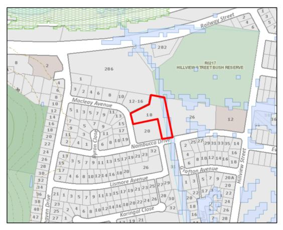
Figure 1 – Extract of GEMS Gosford Electronic Mapping System – 1% AEP Flood Extents
