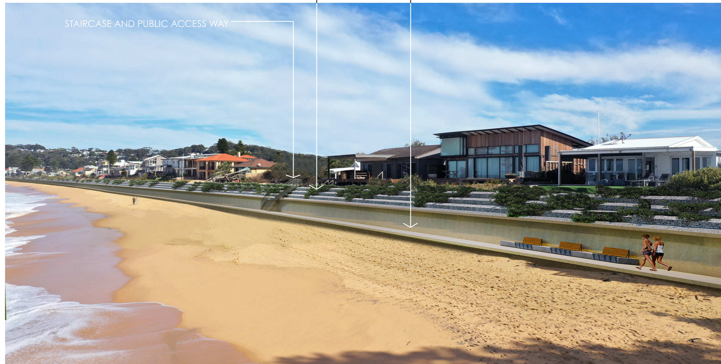
image: concept design option 5 - tiered vertical seawall with promenade (Wamberal Terminal Coastal Protection Assessment, Draft Final Stage 3 - Seawall Concept Design Options, May 2021)
