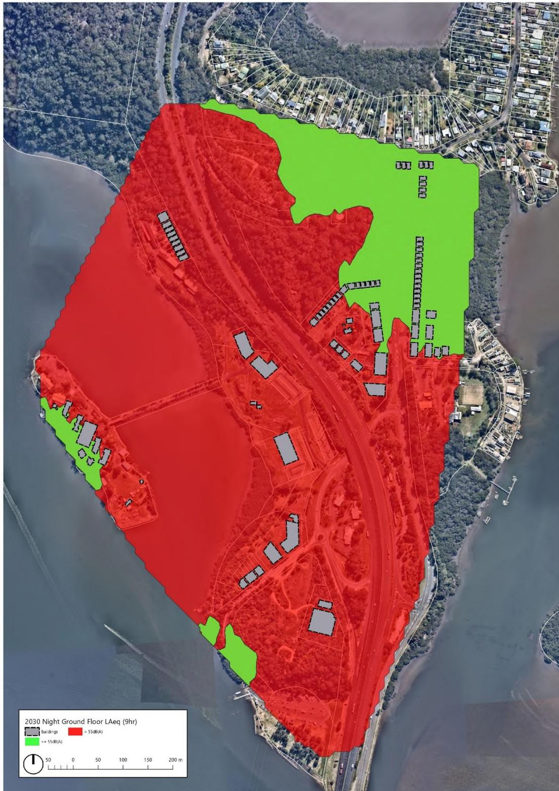
Figure 6 – 2030 Night-time  $L_{Aeq}$  (9hr) Noise Contour (First Floor)
