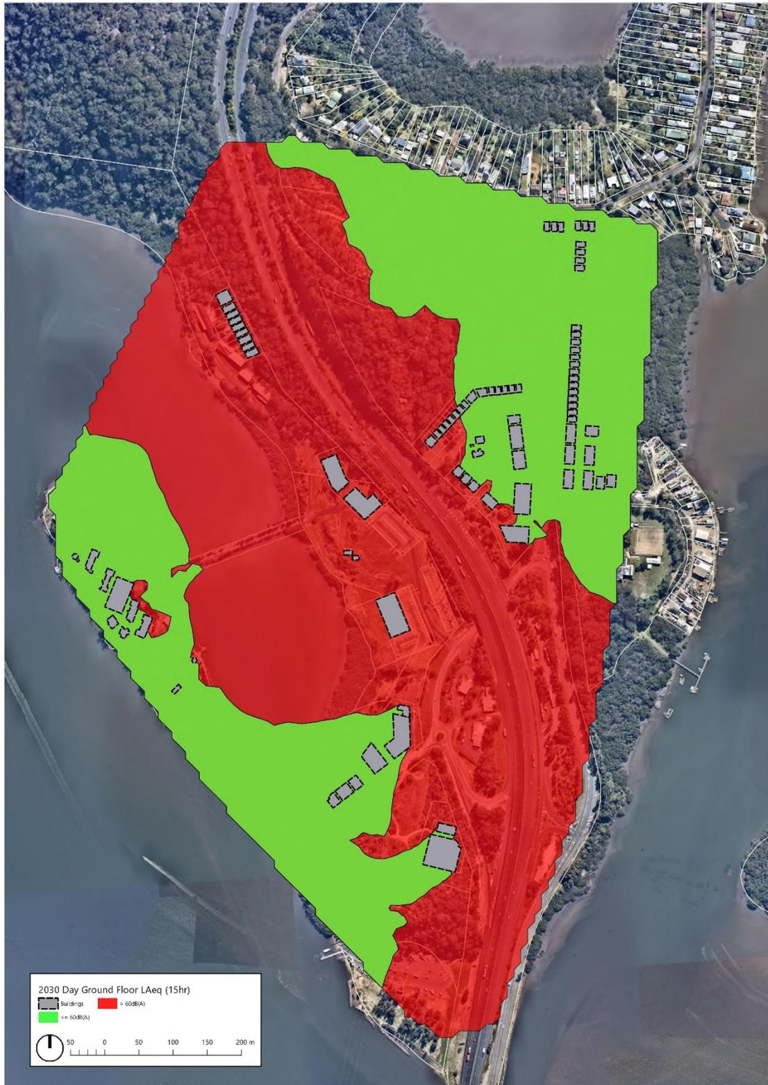
Figure 3 – 2030 Day-time  $L_{Aeq}$  (15hr) Noise Contour (First Floor)
