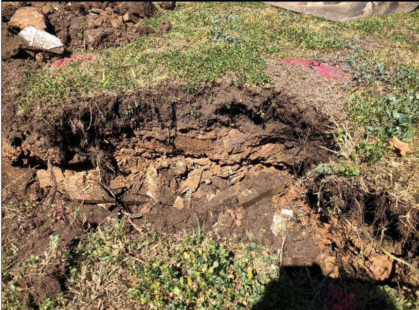
PHOTOGRAPH 11: PORTION 3 – BURIED ASBESTOS IN THE NORTHERN PORTION OF PEAT ISLAND
