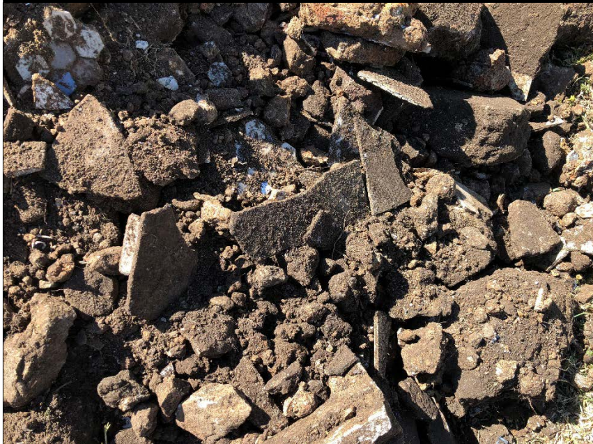
PHOTOGRAPH 12: PORTION 3 – ACM FRAGMENTS IDENTIFIED WITHIN SS03
