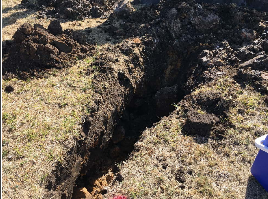
PHOTOGRAPH 12: PORTION 3 – FILL MATERIAL IDENTIFIED WITHIN SOUTHERN PORTION OF PEAT ISLAND
