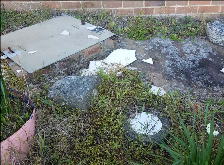
PHOTOGRAPH 3: PORTION 1 - ACM IDENTIFIED ON SURFACE ADJACENT TO VACANT BUILDINGS
