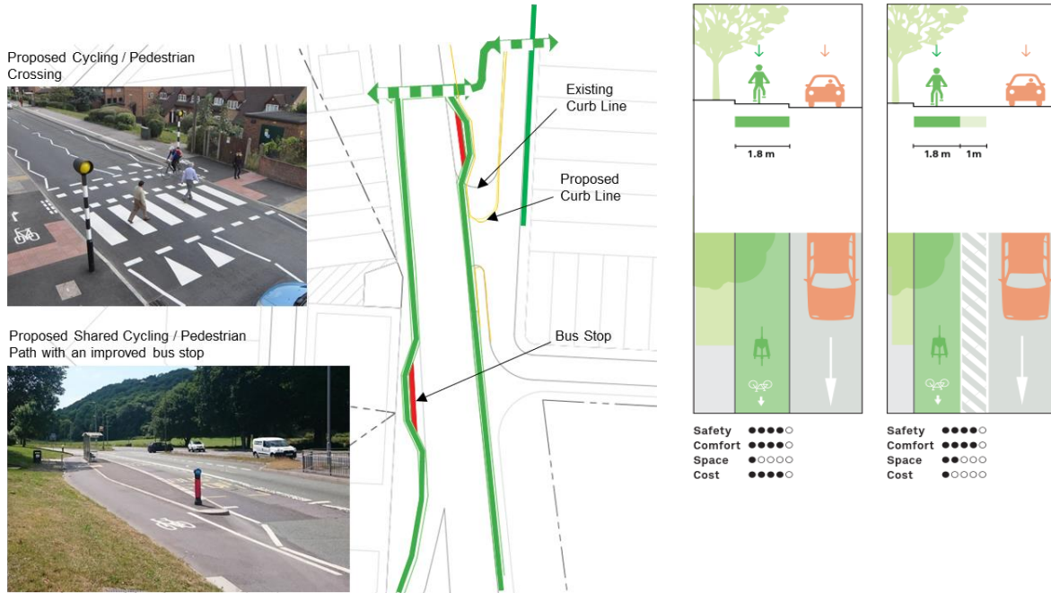
Figure 6.2: Proposed infrastructure around pedestrian connection (left) and concept cross section for dedicated cycle lanes
