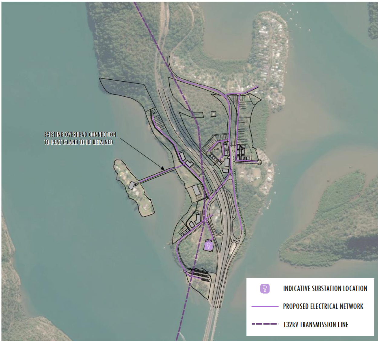
Figure 11: Proposed Zone Substation Location
