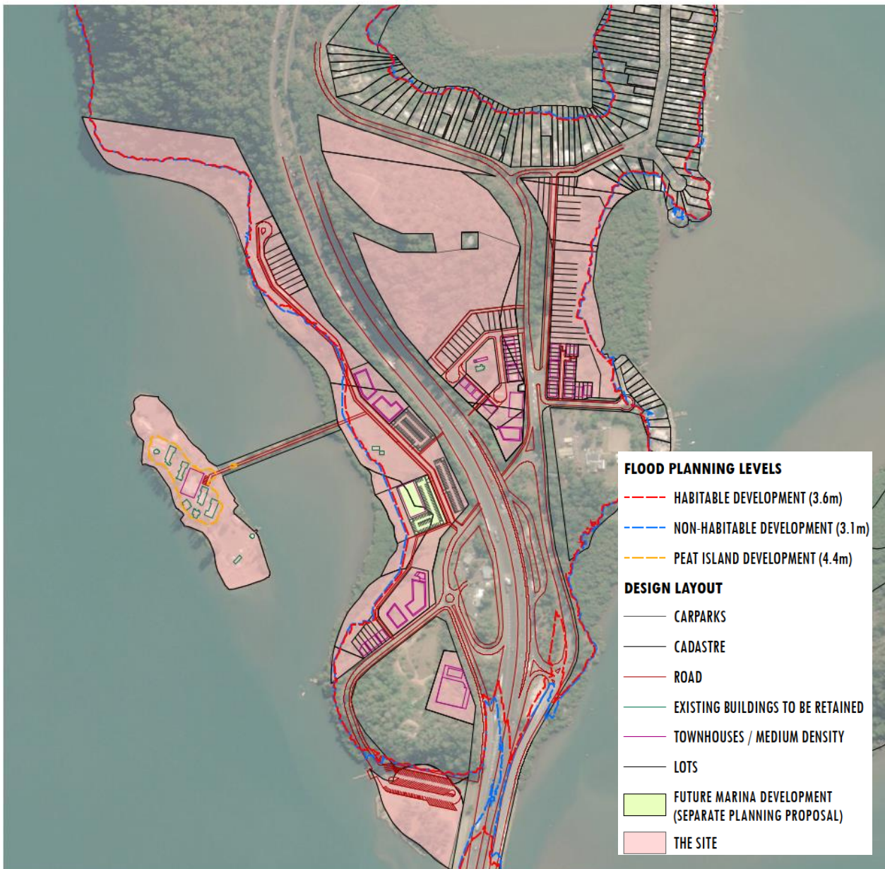
Figure 6: Flood Planning Level
