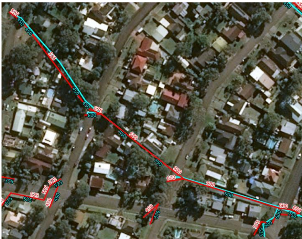
Figure 6.14 – Minor Discrepancies between Council (Blue) and Modelled (Red) Data (Diameters displayed along pipes are in mm) Top Budgewoi; Bottom: Halekulani
