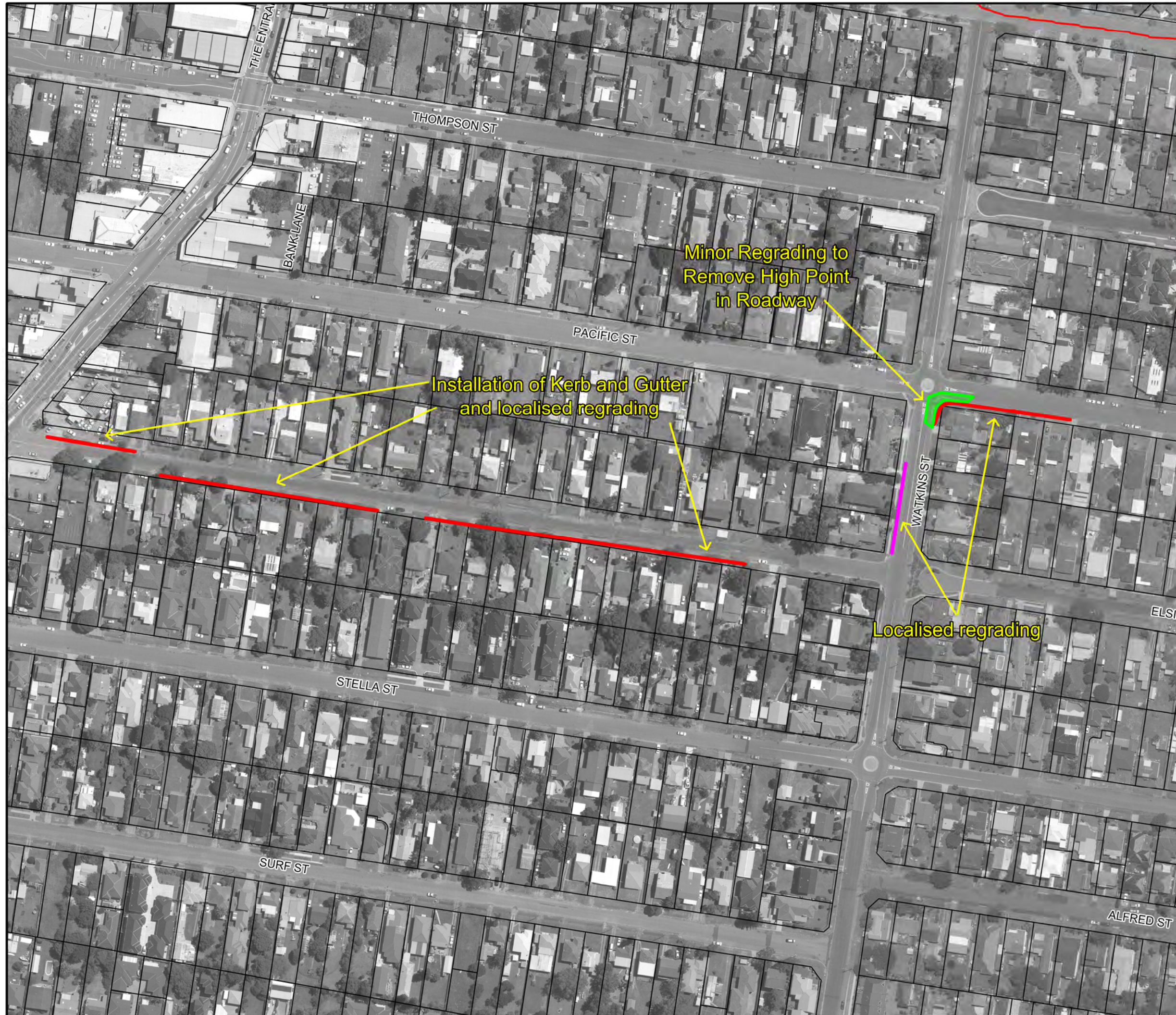
Figure 25 Concept Design for Installation of Kerb and Gutter along Elsiemer St and Pacific St
