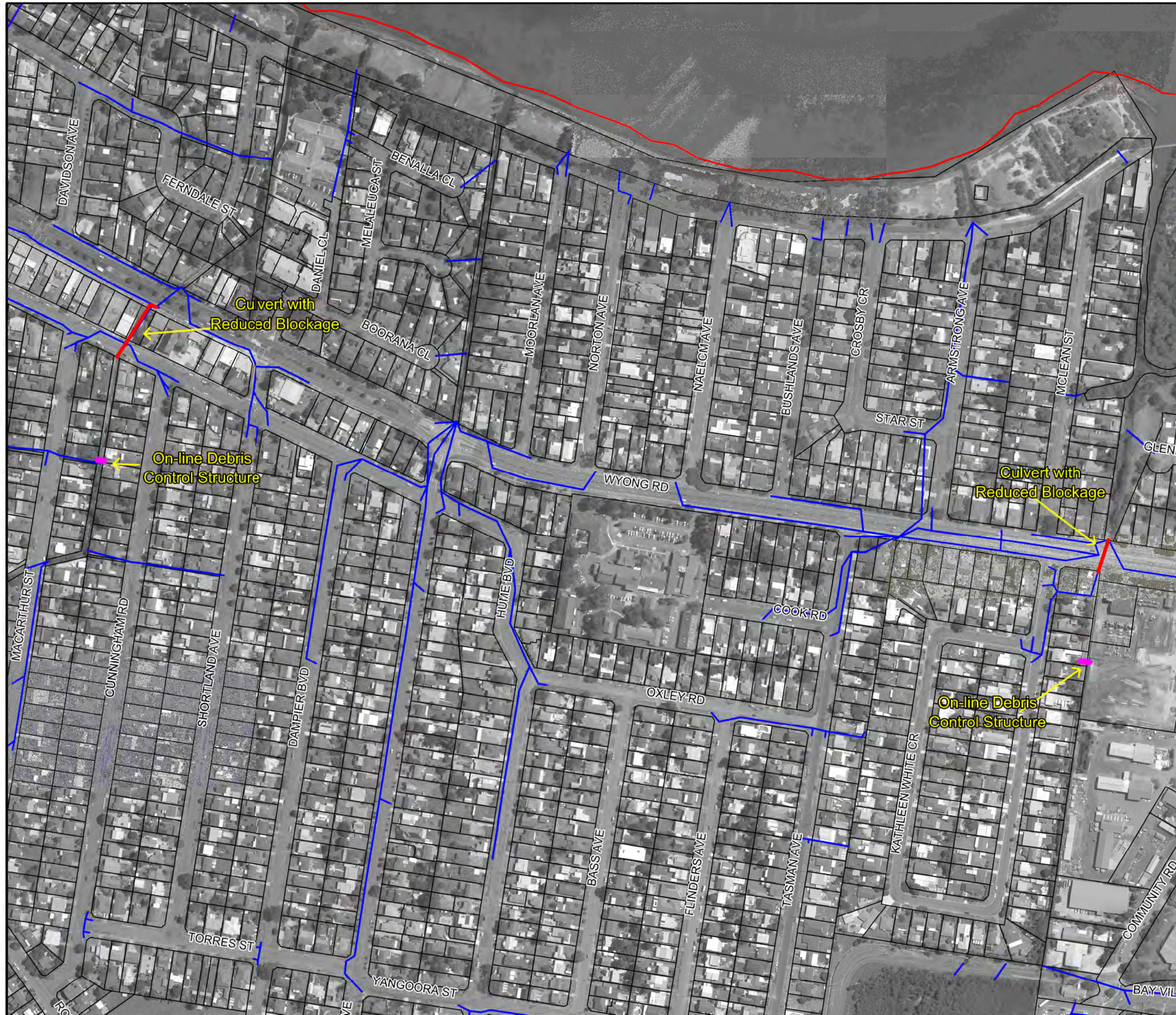
Figure 19 Concept Design for Blockage Control Structures Upstream of Culverts
