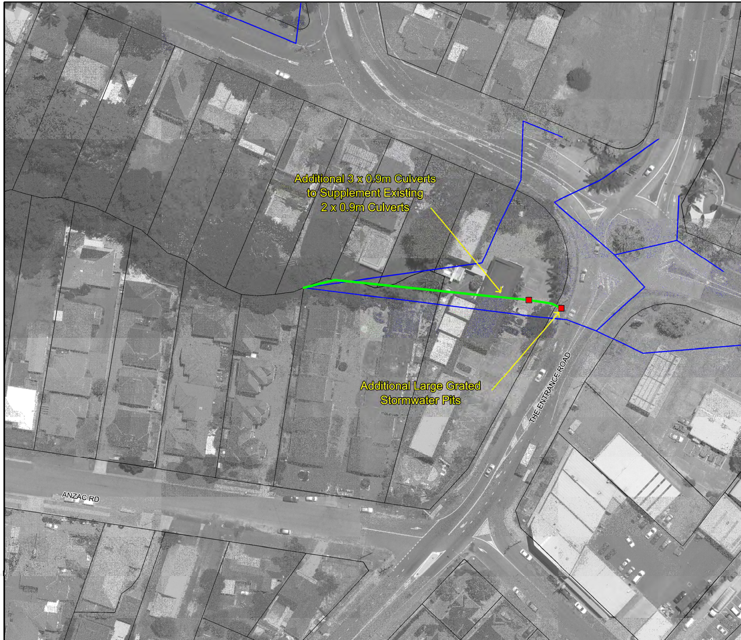
Figure 22 Concept Design for Culvert Upgrade between The Entrance Rd and the rear of The Reef Resort Motel
