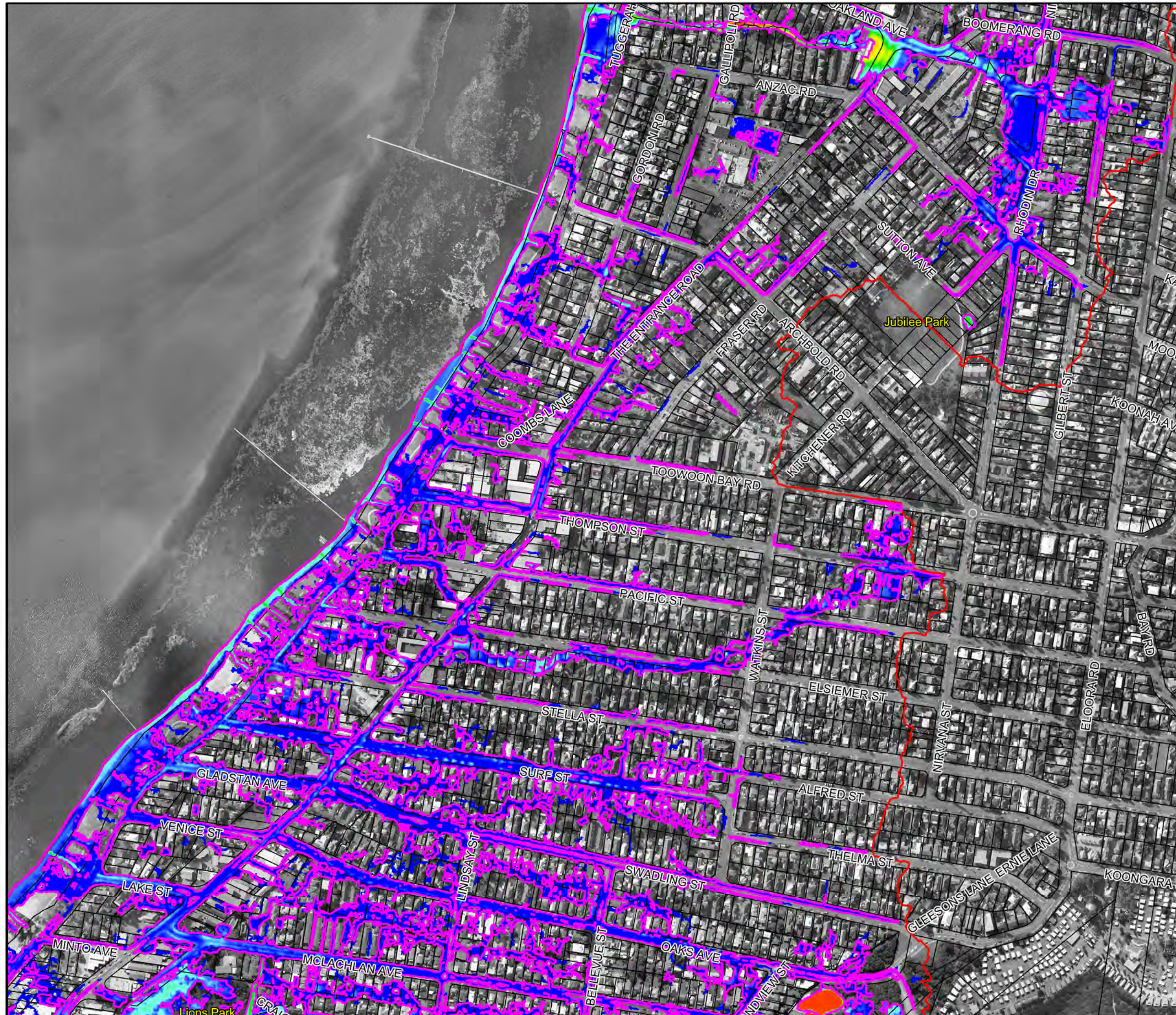
Figure 16.4 Peak Floodwater Depths for the 1% AEP Flood with 18.6% Increase in Rainfall Intensity associated with Climate Change
