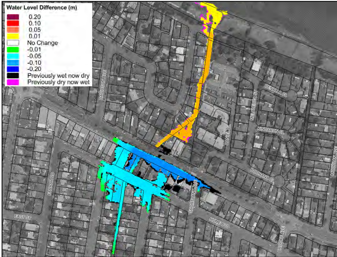
Plate 20 Peak 20% AEP Flood Level Difference Mapping with Culvert Upgrades between Hume Boulevard and Wyong Road
