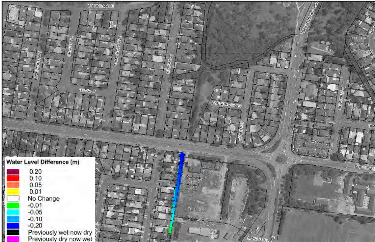
Plate 18 Peak 20% AEP Flood Level Difference Mapping with Culvert Upgrade under Wyong Road near Kathleen White Crescent
