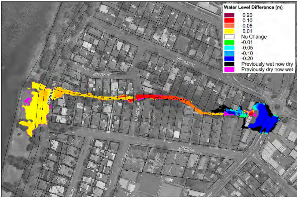
Plate 33 Peak 20% AEP Flood Level Difference Mapping with Regrading across the Reef Resort
