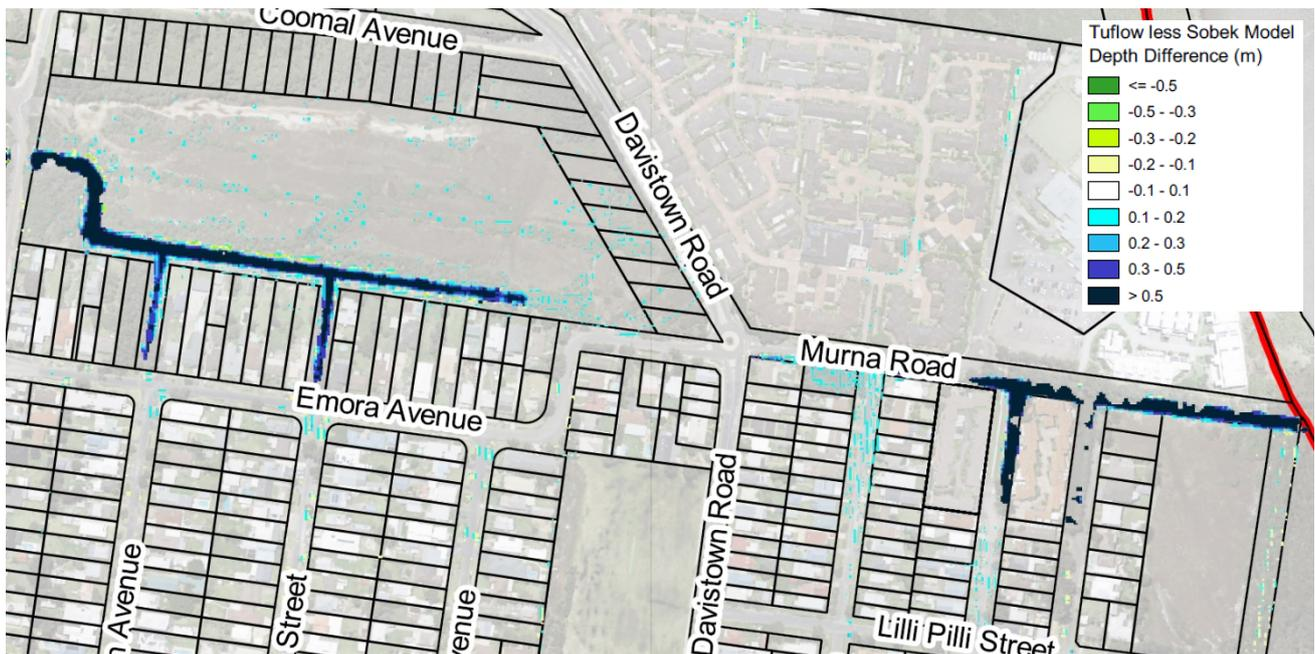
Figure C-11-3 Open Channel Depth Differences - 1% AEP
