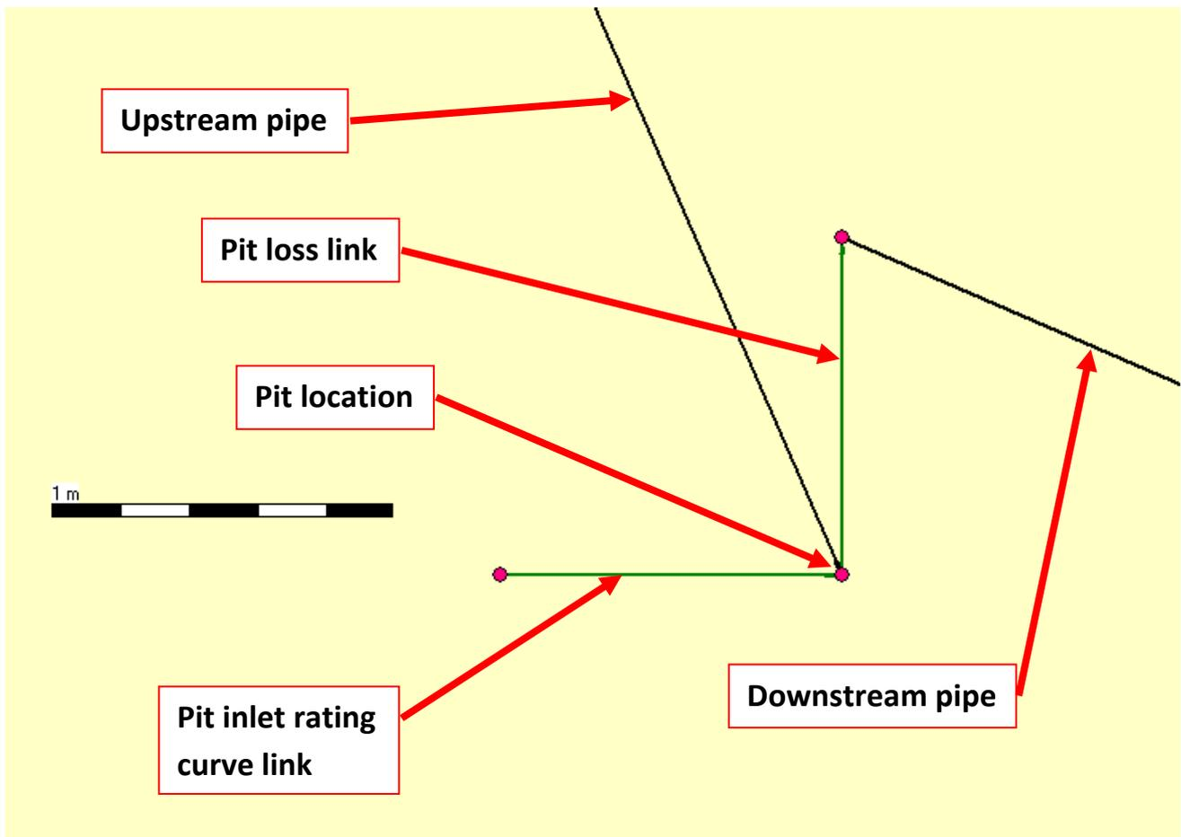
Figure C-11-2 Sobek Model Pit Schematisation
