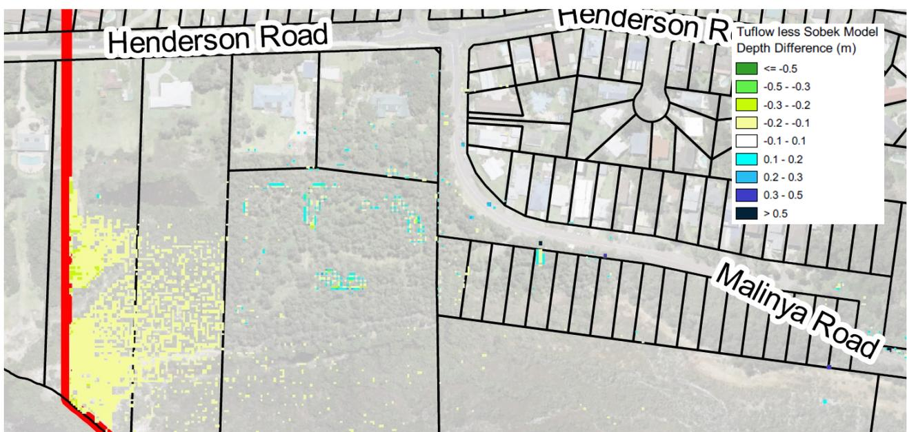
Figure C-11-4 Boundary Conditions Resulting in Depth Differences - 1% AEP
