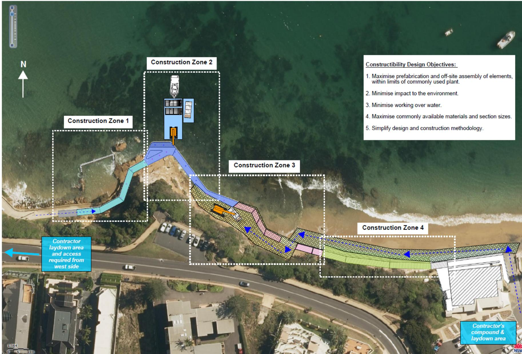
Figure 6: Proposed construction methodology
